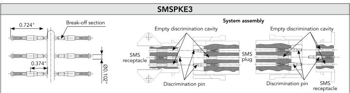
A pin, which can be inserted in the discrimination cavities of the SMS Quick Mating cable and board mount connectors. The discrimination cavities are in between of the contact cavities and offer the advantage that no contact cavities are lost due to discrimination. As extraction tool, the RX2025GE1 without the "extraction tool tip" can be used.
